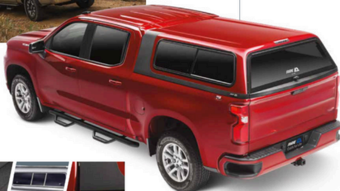
SINGLE T HANDLE OPTIONAL OUTDOORSMAN VENTED WINDOW PACKAGE SPRAY-ON PROTECTIVE COATING INCREASES STRENGTH IN HIGH STRESS AREAS
